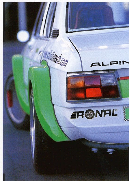
Above. Wide arches are Alpina group 2 parts and just about cover the 13 inch wide rear wheels. Below. Later front grille was fitted by Martini Racing.
