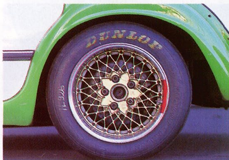
Above. With 10 inch wide BBS split-rims on the front and no power steering or power brakes, the E12 would have been a demanding car to race.
