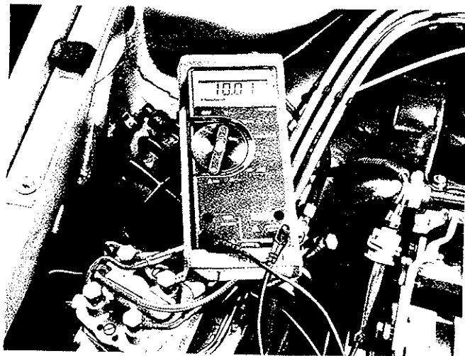
Fig. 6-16. Typical actuator current, engine warm, open-loop (lambda sensor disconnected).
